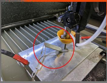
Bend the orange split guard to flip it over. Then move it down so it touches the surface. Also add water to the machine until the material is about 5 mm covered by water.
