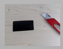
In the meantime cut the vinyl cut the vinyl to rough size using a knife. And peal away the material that you do not want to print.
