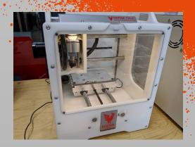
The software will recognize the machine and ask you to home it. Make sure nothing is located on the table and press "Start Homing..."
