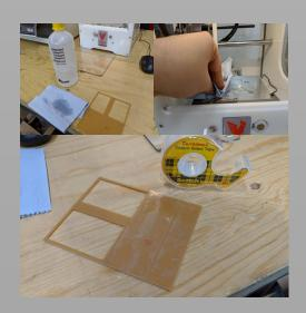
Place your material on the table. Make sure it is aligned with the front left corner of the bracket.
