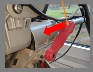
Adjust the bevel angle using the bevel angle scale
