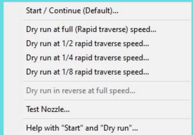
During the dry run check that there are no collision. You can see the progress on the screen. After the dry run is done use the [Go Home] button to get back to the correct starting position.
