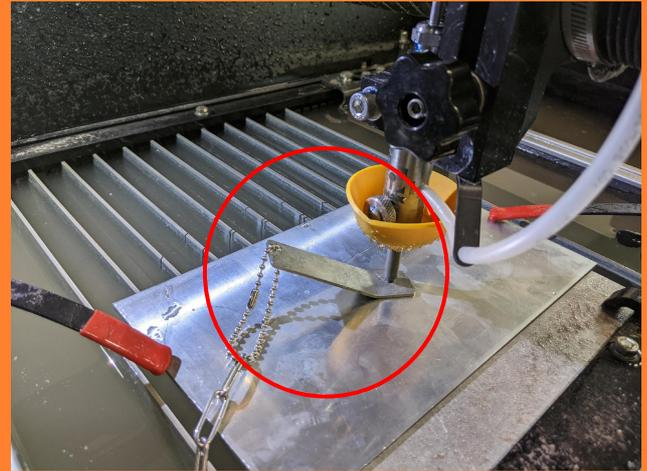
Bend the orange split guard to flip it over. Then move it down so it touches the surface.
