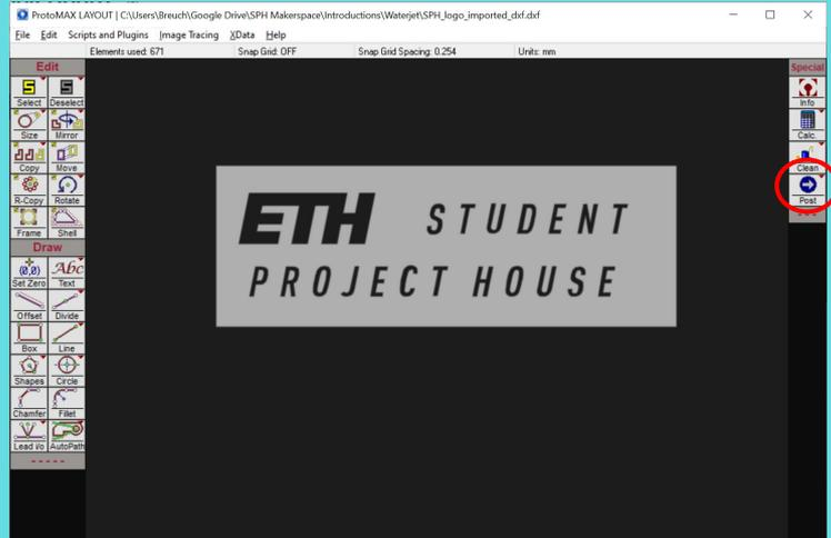
Select the starting point. The point must be an end point. Make sure to always use the point so that the inner parts are cut first.
