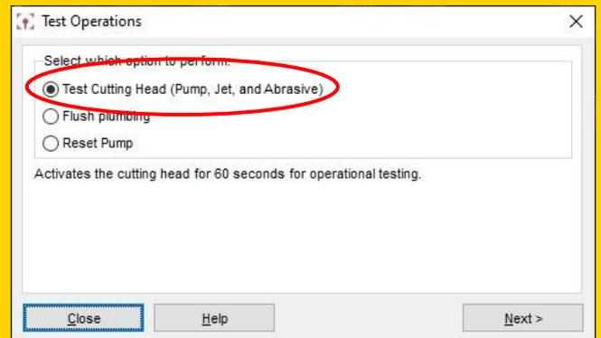
Double check that the abrasive tube is removed and secured, and that the cutting unit is between two slots. Then press [Start Test].
