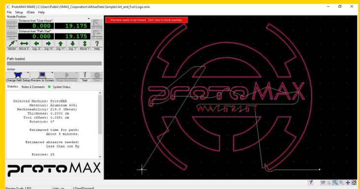
The machine will move around. Make sure that it will not hit anything. Once the machine is done the window on the right is shown.
