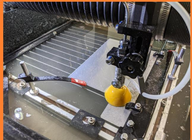
Add water to the machine until the material is about 5 mm covered by water.
