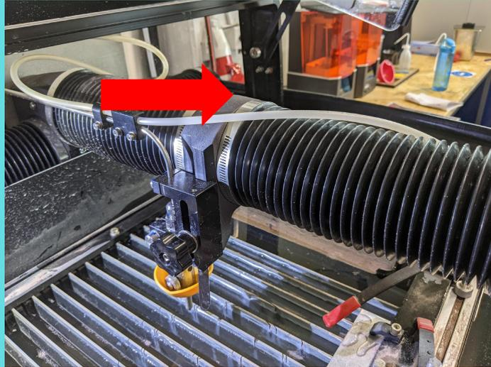
Release the head unit and move it to about 5 mm above the metal slats using the big black knob. Make sure that the head unit does not crash into the slats.
