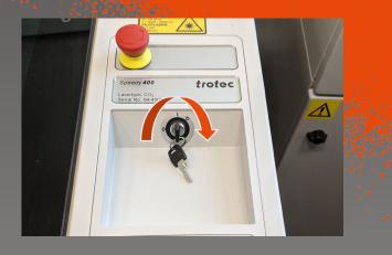
The machine will run several self checks and calibrate the axis. This process will take a few seconds and will cause the table to move all the way down.
