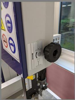
The blade guard can be adjusted on the right.
