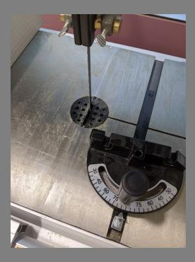
The push guide can be used to cut parts flat perpendicular to saw.
